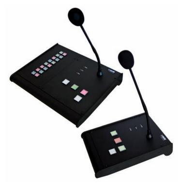
The base Paging Station with 4 configurable push buttons can be fitted with 16-button extension modules. This allows to create Paging Stations with 4, 20, 36, 52 or 68 push buttons.
